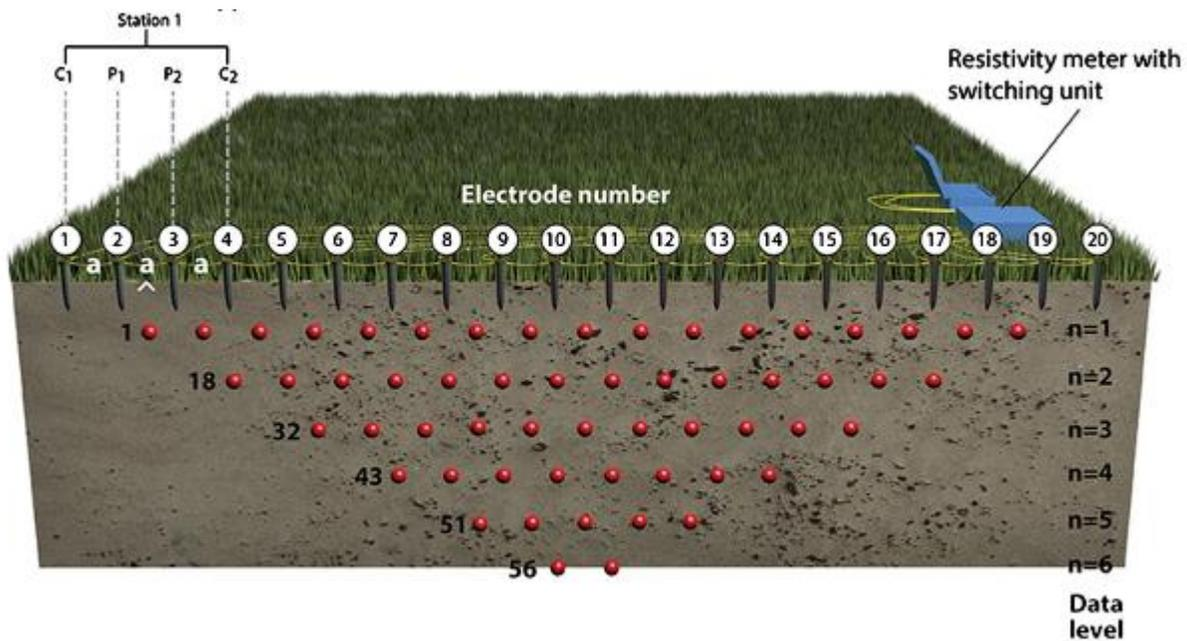
Schematic diagram: A multi-electrode system, and a possible sequence of measurements to create a 2-D pseudo section.
