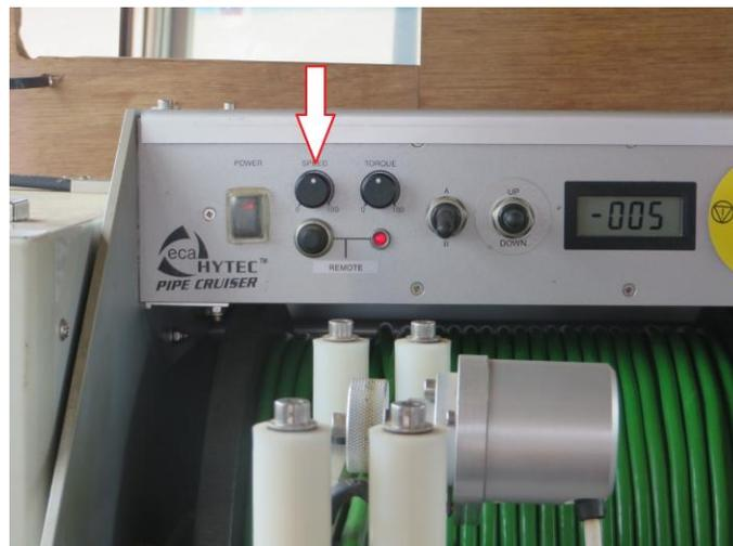
18- Keep on pressing on the down button till reaching the bottom of the borehole
