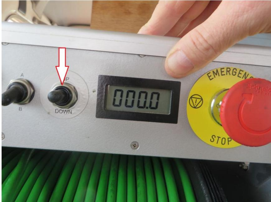
17- Calibrate the speed of the cable using the speed button on the winch to achieve 4m/min cable speed. This speed is used both for static as well as for dynamic mode. However in dynamic mode we also take readings at 6m/min that why it's important to write the speed of the cable while saving your file as explained in point number 14.
