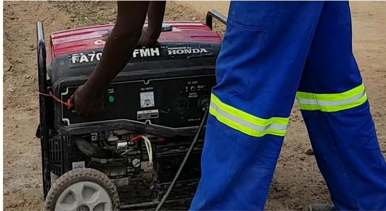
12- Switch on the electrical board once the generator is on.
