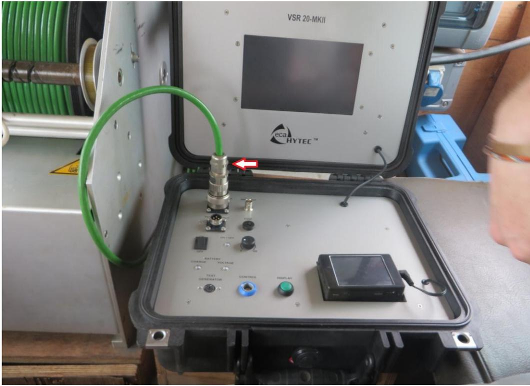
8- Connect the TV monitor to the control unit VSR20 MKII and to the power supply
