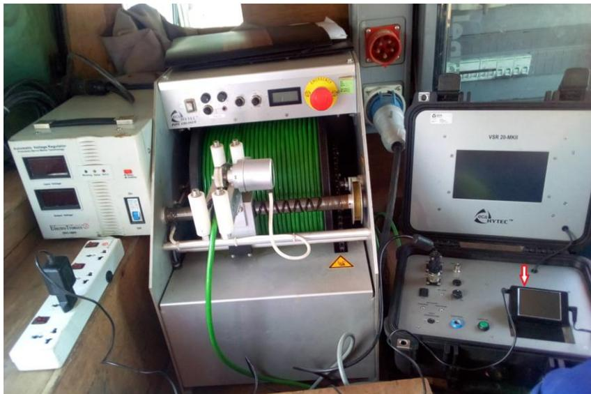
7- Connect the back umbilical cable of the winch to the control unit VSR20 MKII.
