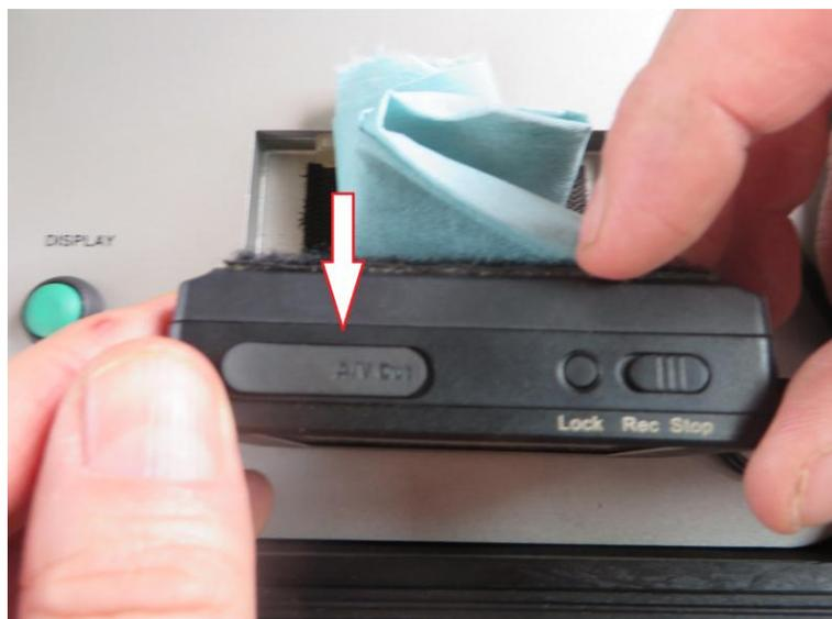
15- Switch off the video recorder by pressing the side on/off button.
