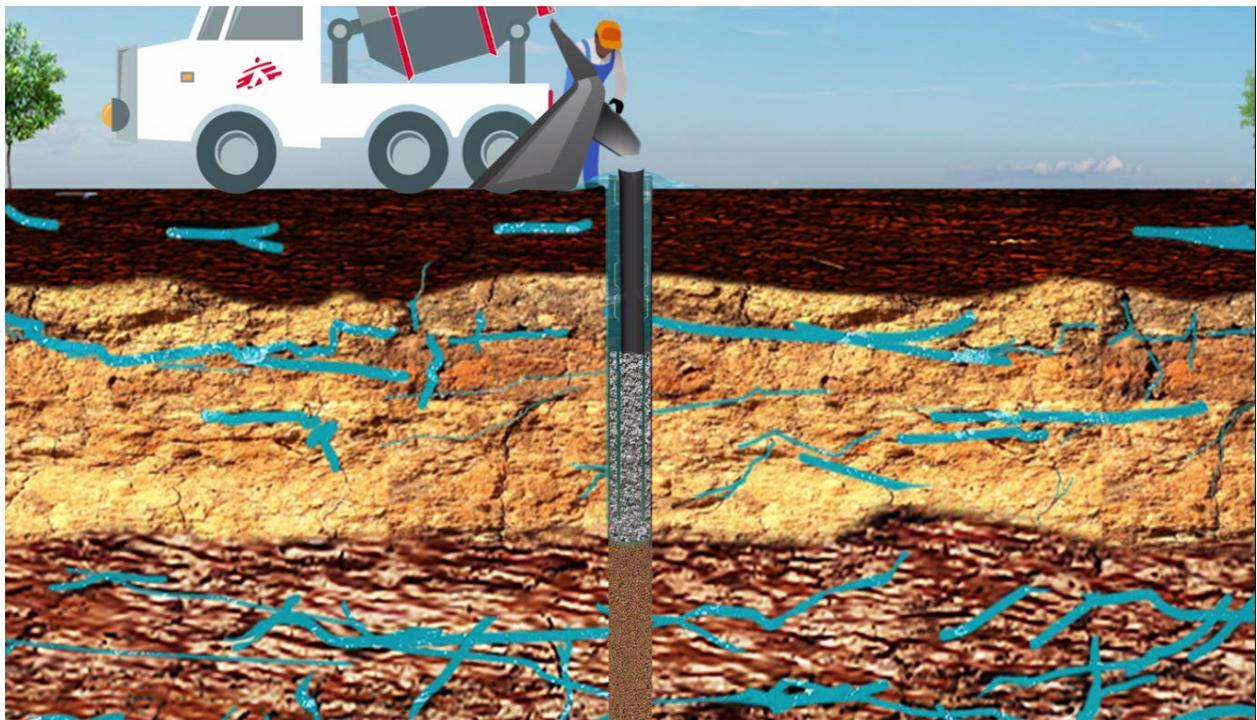
Figure 19: Animation shows how grout is settled at the bottom of the hole
