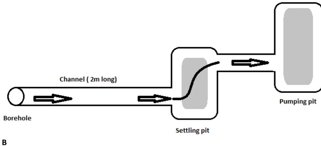
Figure 2: Mud Circulation: A: Plan View; B: section view
