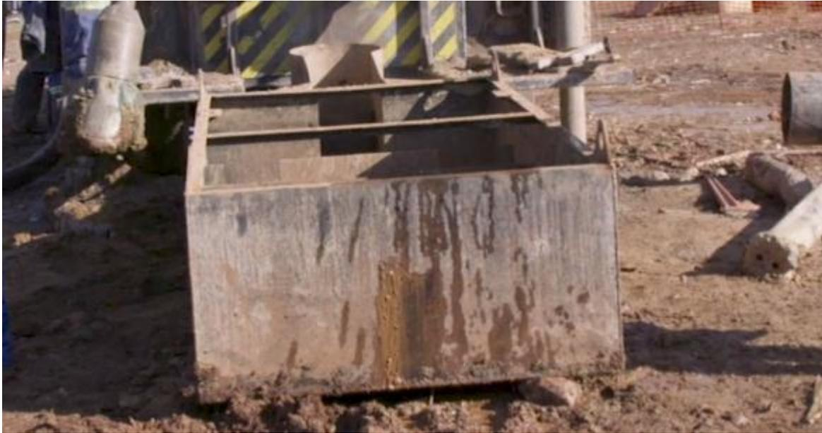
**Figure 3: Mud pan for mud rotary drilling**
