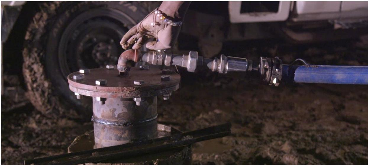
**Figure 22: Closing of flange valve to maintain the pressure**
