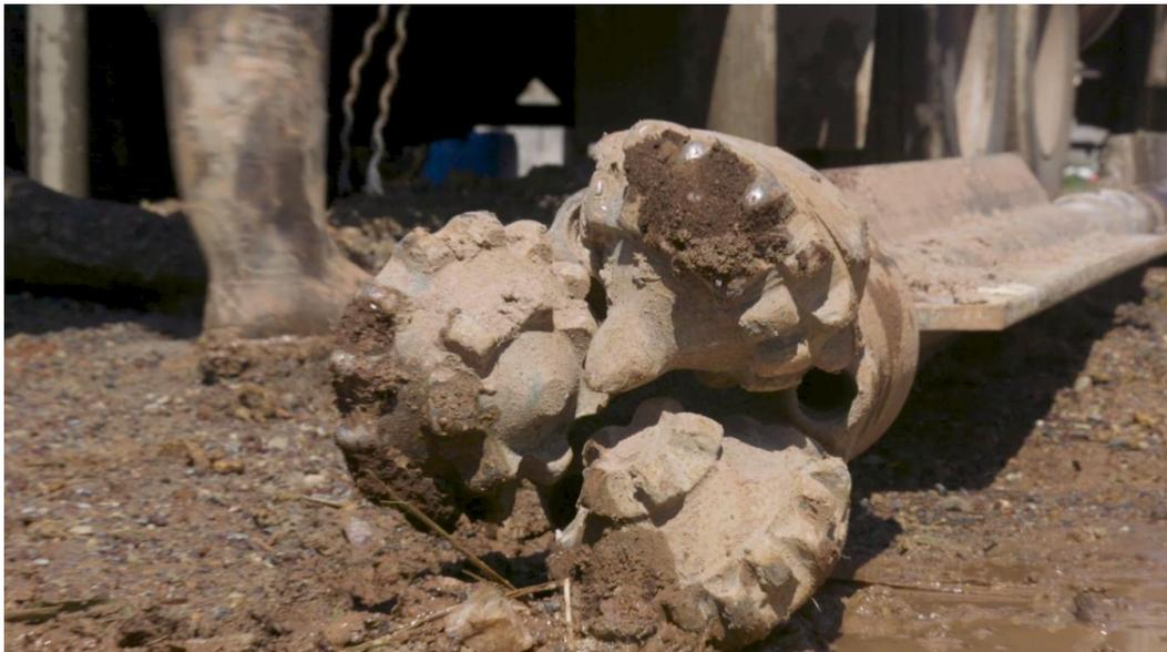
**Figure 1: 260 mm tri-cone drill bit used for mud rotary drilling in top unconsolidated formations**
