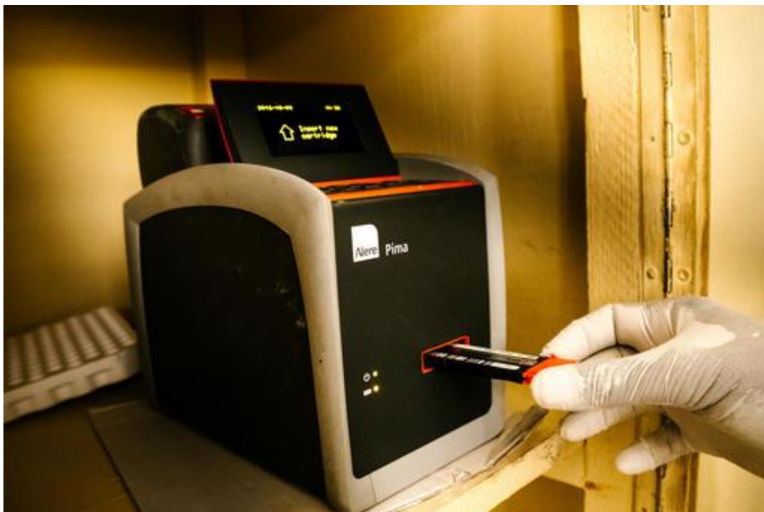
A PIMA point-of-care CD4 test device used in an MSF advanced HIV disease programme in Nsanje, Malawi. Photo: Isabel Corthier/MSF
