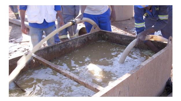
Figure 8: Circulation of drilling mud inside the mud pan to keep the mixture homogenous before drilling
