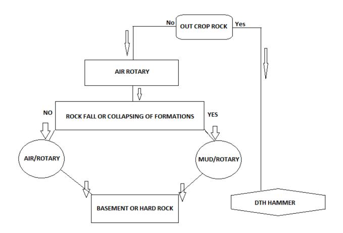
Figure 5: Flow chart for selection of drilling technique
