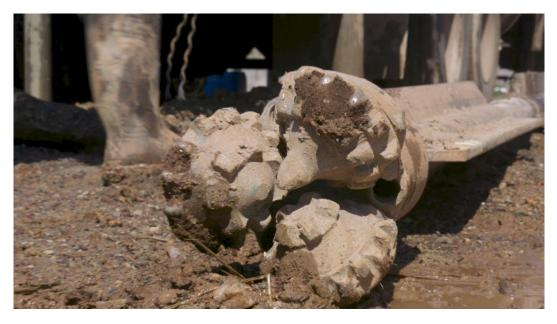
Figure 1: 260 mm tri-cone drill bit used for mud rotary drilling in top unconsolidated formations
