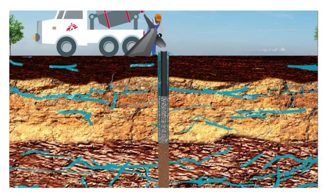
Figure 19: Animation shows how grout is settled at the bottom of the hole
