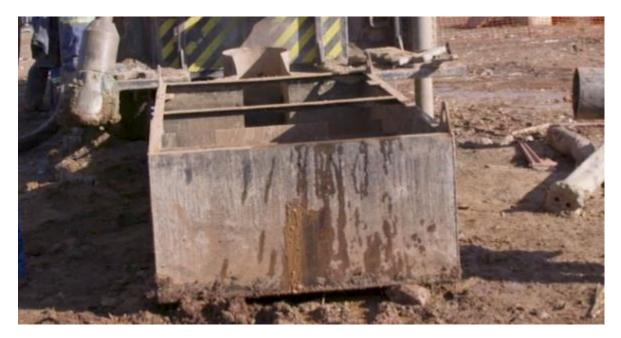
Figure 3: Mud pan for mud rotary drilling
