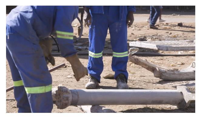
Figure 4: 6.5" DTH hammer drill bit attached to a drill rod
